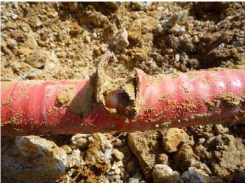
Damage to insulation cable by tent peg or spike
