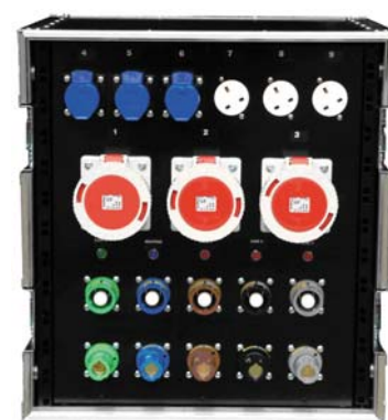
Fig 5: A distribution unit consisting of: Incoming: 400A Power lock with link through Outgoing: 3 x 63A, 3Ø, to BS EN 60309-2 3 x 16A, 1Ø, to BS EN 60309-2 3 x 13A, 1Ø, to BS 1363
